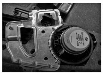
At the original metal sheet, on which the midrange speaker is installed, the fold (see picture) has to be face grinded, that the **GLADEN** midrange speaker rests on the metal sheet.
